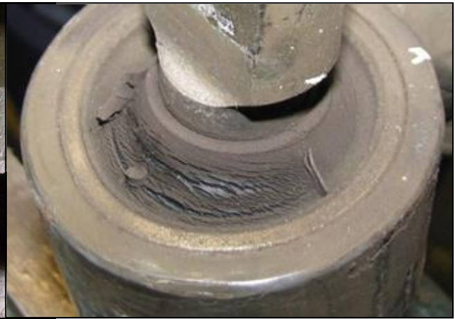
Figure 5-3; Acceptable surface cracks
